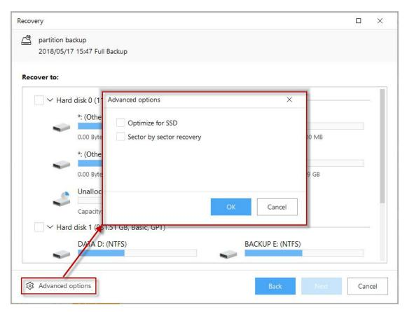
Optimize for SSD - If the destination disk is SSD, check this option will ensure sector alignment in the process.
