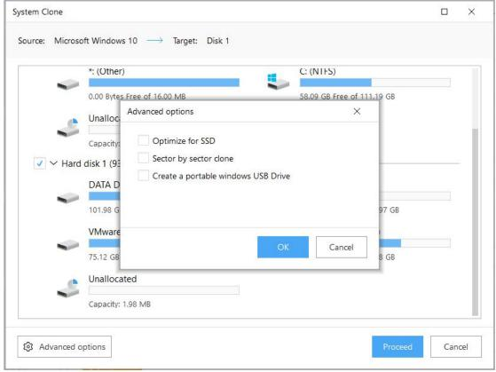
Please make sure the capacity of the unallocated space on your target drive is larger than the total size of your boot and system partition. "**Optimize for SSD**" is highly suggested if your target drive is an SSD. Please check the "**Create a Portable Windows drive**" option if the target disk is connected via USB.
